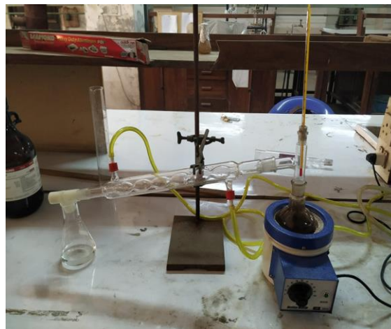
Fig. 2: Separation of ethanol and anthocyanin by bulb-type condenser
