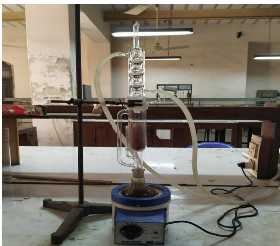
Fig. 1: Soxhlet extraction of H. rosasinensis
