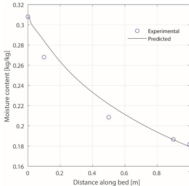
Fig. 5 Comparison between experimental and predicted moisture content along the bed length.  $u_g = 3$  m/s,  $T_{g,0} = 373.15$  K,  $Y_0 = 0.0018$  kg/kg,  $S = 0.0041$  kg/h,  $X_0 = 0.308$  kg/kg,  $T_{s,0} = 301.15$  K,  $v = 0.005$  m/s.
