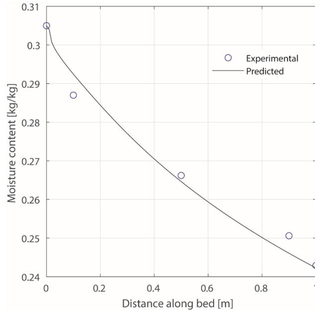
Fig. 4 Comparison between experimental and predicted moisture content along the bed length.  $u_g = 3$  m/s,  $T_{g,0} = 343.15$  K,  $Y_0 = 0.0010$  kg/kg,  $S = 0.0094$  kg/h,  $X_0 = 0.305$  kg/kg,  $T_{s,0} = 301.15$  K,  $v = 0.008$  m/s.
