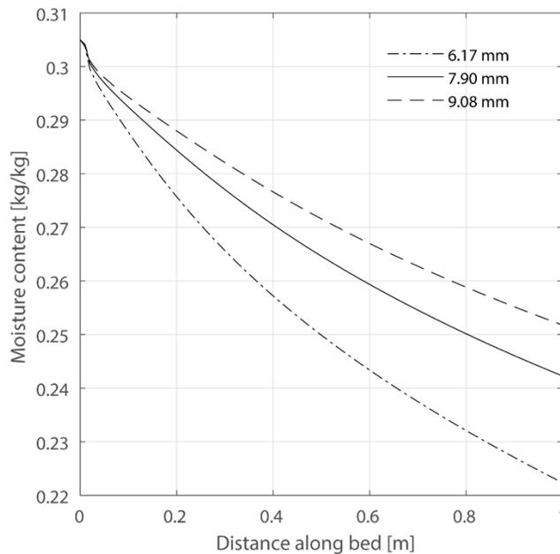
Fig. 7 Effect of particle size on drying behaviour.  $u_g = 3$  m/s,  $T_{g,0} = 343.15$  K,  $Y_0 = 0.0010$  kg/kg,  $S = 0.0094$  kg/h,  $X_0 = 0.305$  kg/kg,  $T_{s,0} = 301.15$  K,  $v = 0.008$  m/s.
