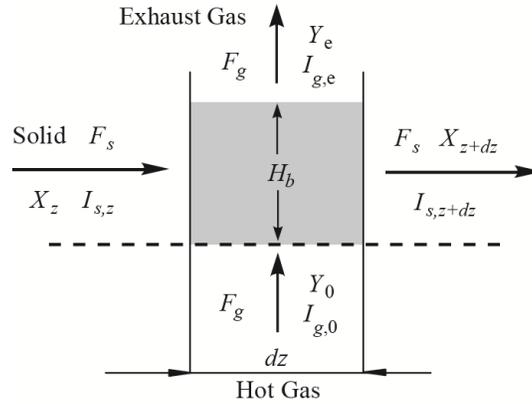
Fig. 2 Scheme of a differential dryer element.
